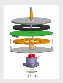
Single-rotor, iron-coreless direct drive motor in which the stator has no core and eliminates the rotation irregularity called cogging. Sophisticated control of the drive motor's rotation speed to ensure highest stability, utilizing the latest motor control technology refined through the development of Blu-ray disc player products
