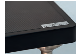
CARBON FIBER / GLASS FIBER / KRION / MDF MULTILAYER PLATFORM Carbon fiber 100% 3K Twill 200gr/m 2 on both upper and lower faces, with G10 biaxial glass fiber 180 gm/m 2 inner core. Finishing like fiber arms.
