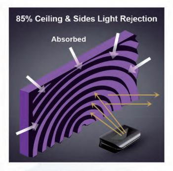
With Fresnel Lens Technology, the screen can absorb 85% of overhead and side ambient light, direct the incident light towards the audience to increase image quality and contrast.
